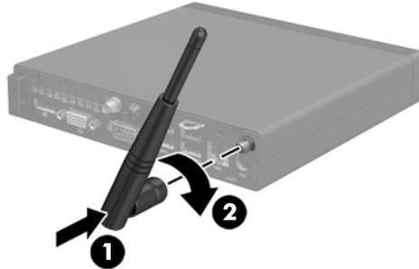
19. Connect the external antenna cables to the WLAN module.
