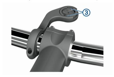
7 Press down slightly and turn the Edge device clockwise until it locks into place.
