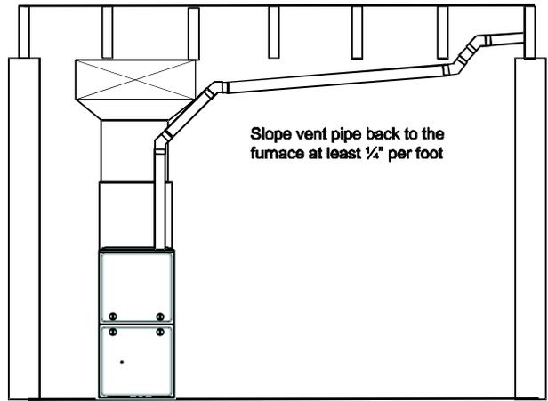
Slope vent pipe back to the furnace at least 1/4" per foot
