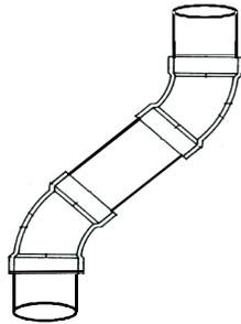
Use 45 deg. Elbows where possible, to ensure condensate drainage.
