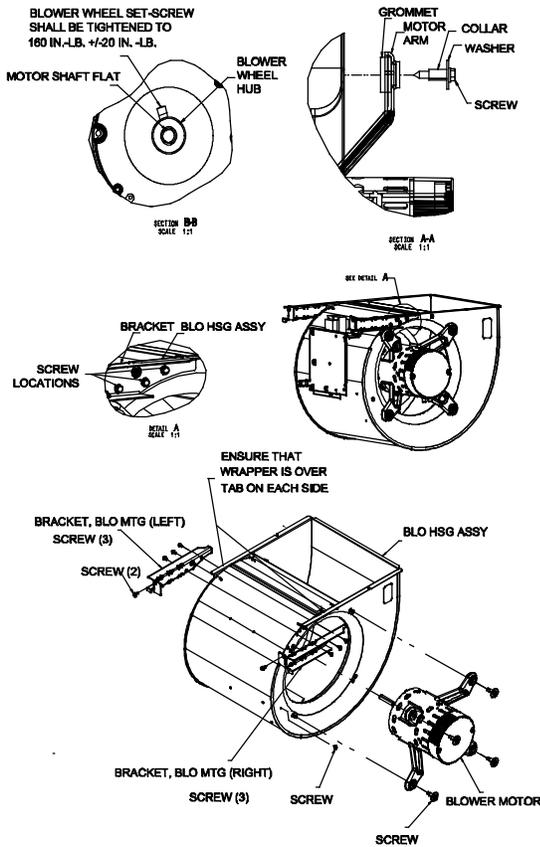
Fig. 67 - Blower Assembly on 100E21-22
