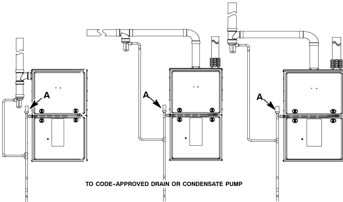
Recommend "T" fitting with 4-inch minimum height standpipe (A) of same diameter or larger extending upward.
