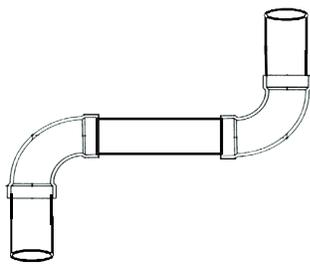
Avoid short horizontal offsets with 90 deg. Elbows. Short offsets can be difficult to slope and may trap condensate.
