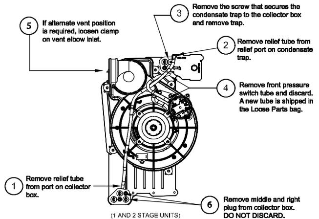
Unconverted Factory Trap Configuration
