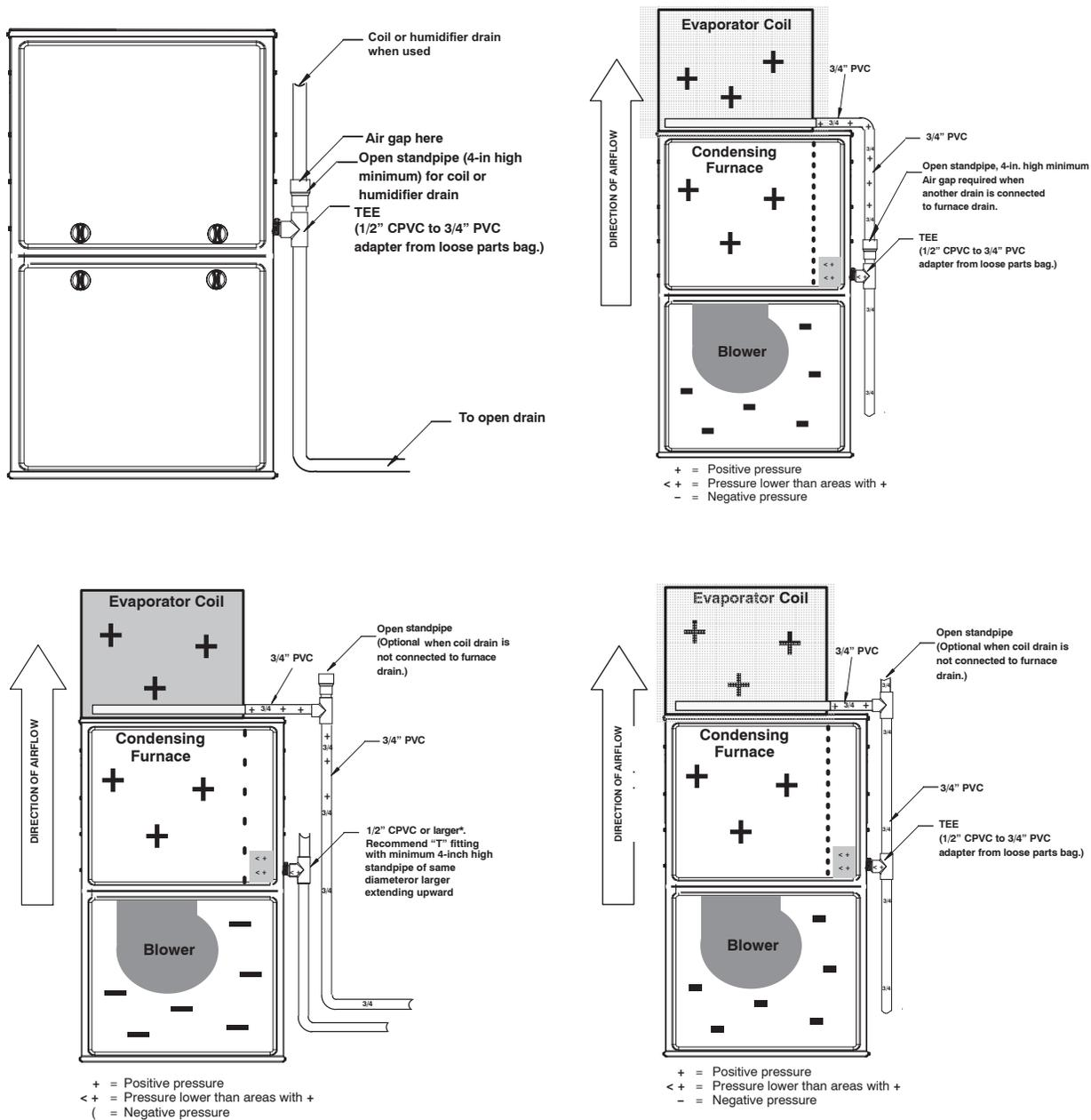
Fig. 12 - Example of Field Drain Attachment
