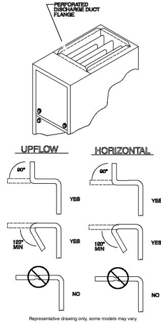
Fig. 20 - Duct Flanges
