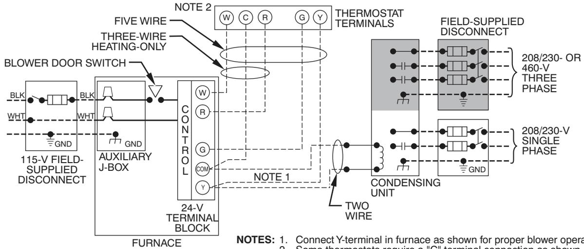
**NOTES:** 1. Connect Y-terminal in furnace as shown for proper blower operation.
