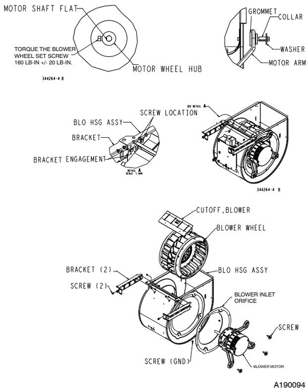
Fig. 66 - Blower Assembly on 040E14-10 and 060E14-12
