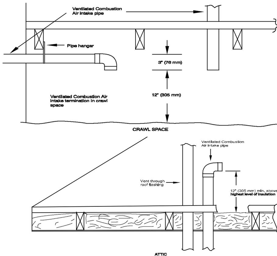
Fig. 47 - Vent Terminations for Ventilated Combustion Air
