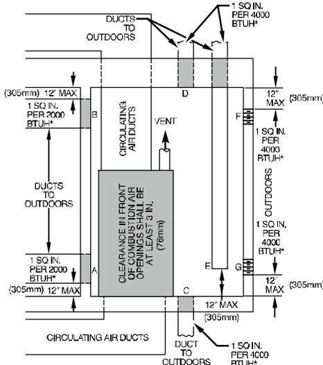
\*Minimum dimensions of 3-in. (76mm)
