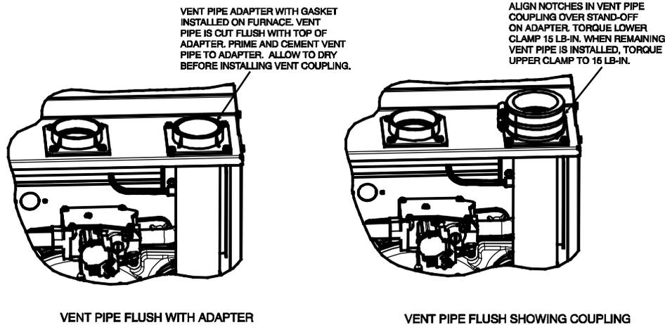
Fig. 59 - Optional Vent Pipe Flush with Adaptor
