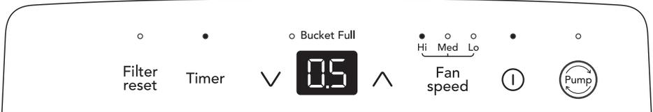
7. Press PUMP button, the unit will enter water pump mode. Pump Mode Indicator will be on. When the water tank is full of water, the pump will start to pump water automatically. The pump will stop automatically after the water tank has been empty.
