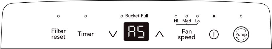
2. If the display reads "EC", check the following operating conditions. Outlet voltage should be 115V±10% and the surrounding temperature should be with in the range of 41 °F to 89 °F. Unplug the unit and plug it in again under normal operating conditions. If the "EC" code persists, contact your Authorized Frigidaire Service Center.
