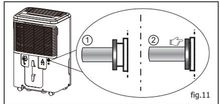
To remove pump drain hose:
