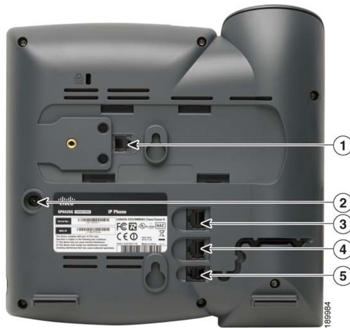
Figure 2 Cisco SPA525G and SPA525G2 IP Phone Connections
