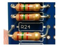
Push or pull the resistors down flush to the board and bend the leads on the backside to hold them in place while soldering.
