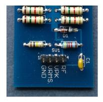
Install C1 the 0.01uF capacitor in the location marked on the board.
