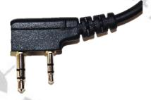
Thus, an external speaker needs to have a 2.5mm TRS-plug with its ring not being connected. The +5V line of the K1 socket is not capable of driving any electronics.
